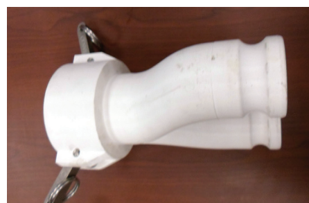
The new Y-shaped design in ABS material wasn't tough enough and cracked during use.
